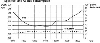
$\textbf{Test conditions} \ \text{Air temperature} \ + 25 ^{\circ} \text{C.} \ \text{Barometric pressure 100 kPa (750 mmHg)}. \ \text{Humidity 30 \%}. \ \text{Diesel fuel}$ acc. to ECE R 24 Annex 6. Density of fuel 0.840 kg/dm³. Viscosity of fuel 3.0 cSt at 40°C. Energy value 42700 kJ/kg. Power test code ISO 3046. Power and fuel values +/-3%.
