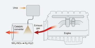
The principle for Scania SCR system
