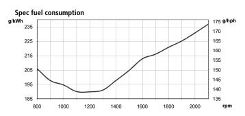
Test conditions Air temperature +25°C. Barometric pressure 100 kPa (750 mmHg). Humidity 30 %. Diesel fuel acc. to ECE R 24 Annex 6. Density of fuel 0.840 kg/dm². Viscosity of fuel 3.0 cSt at 40°C. Energy value 42700 kJ/kg. Power test code ISO 3046. Power and fuel values +/-3%.
